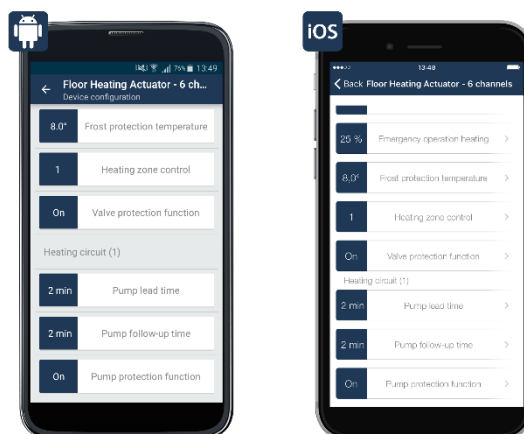
Device configuration Alpha IP Base Station (floor heating actuator)
