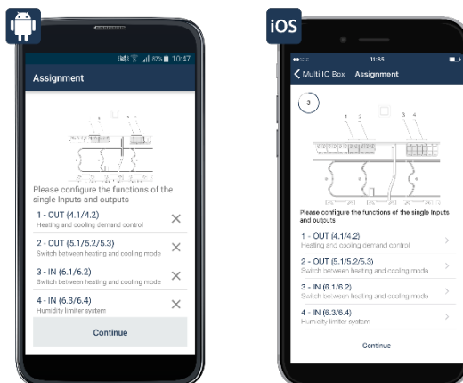
Screenshot: Channel overview, configuration of Multi IO Box for humidity limiter
